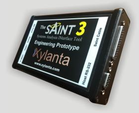
The Xylanta SAINT3 family are the latest generation of products derived from the highly successful SAINT serial communications analysis tools originally developed by Delphi/Aptiv. These new products enhance the SAINT2 design by adding support for CAN-FD in addition to CAN 2.0B, whilst maintaining a high level of software and hardware compatibility with the older product.
