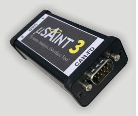
The Xylanta SAINT3 family are the latest generation of products derived from the highly successful SAINT serial communications analysis tools originally developed by Delphi/Aptiv. These new products enhance the SAINT2 design by adding support for CAN-FD in addition to CAN 2.0B, whilst maintaining a high level of software and hardware compatibility with the older product.
